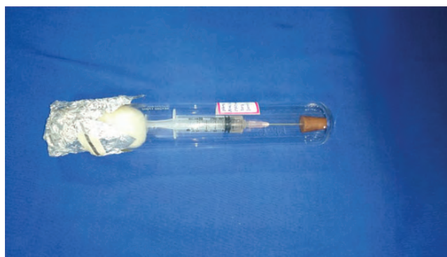
Figure 3. The sterile test tube container used to transfer the sample (aqueous/vitreous/others) to microbiology laboratory.
