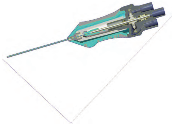
Fig. 2. Dual actuation lines (ALCON) allows duty cycle control, to make cutting more effective
